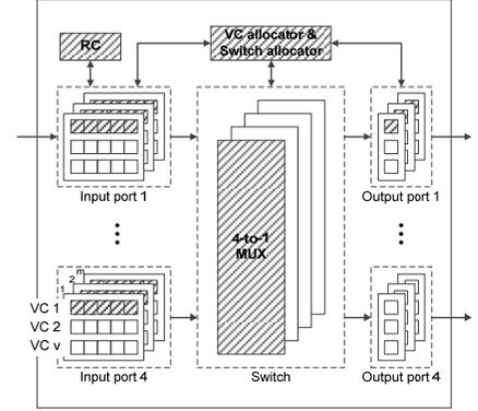
Figure 5: Partially-on design for saving energy while maintaining minimal forwarding functions.
