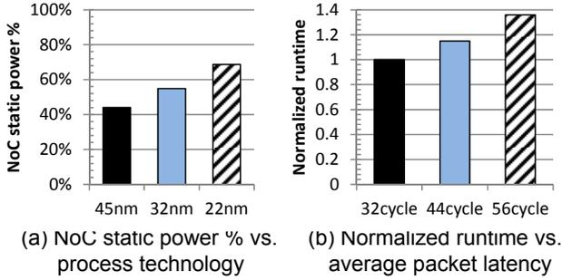
**Figure 1: Need for reducing NoC static power without increasing packet latency.**
