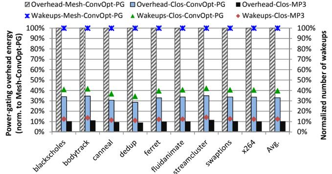
Figure 9: Comparison of power-gating overhead.
