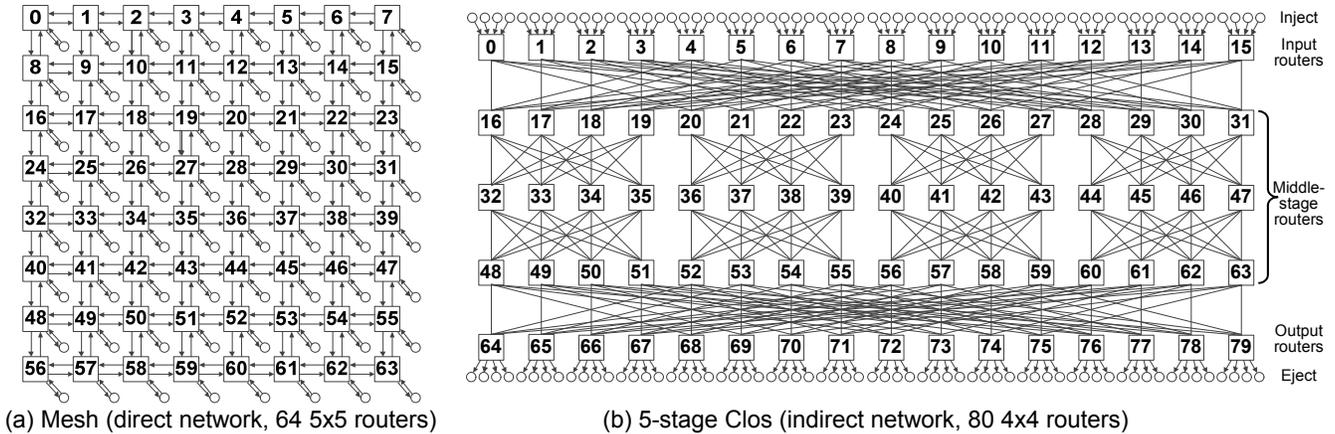
**Figure 3: Direct network (mesh) vs. indirect network (Clos) for connecting 64 PEs; all links are unidirectional. PE-router dependence only at input and output routers in indirect networks.**
