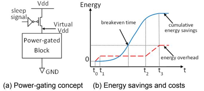
**Figure 2: Power-gating technique and breakeven time.**
